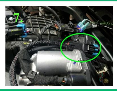
CONNECT REVERSE LIGHT PLUG INTO OEM WIRE CONNECTOR. SECOND PLUG CONNECTS TO LIGHT BAR WHICH IS MOUNT JUST UNDER THE REAR BED.
