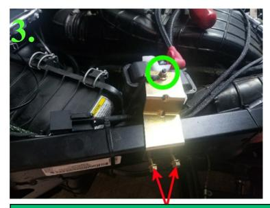
INSTALL BRONZE BRACKET BACK IN ORIGINAL LOCATION. TIGHTEN UP TWO 10MM BOLTS AND REINSTALL COIL PACK CONNECTOR
