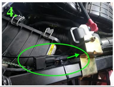
ZIP TIE RELAY TO THE FRAME AND RUN WIRING UNDERNEATH BRONZE BRACKET TOWARD THE REAR
